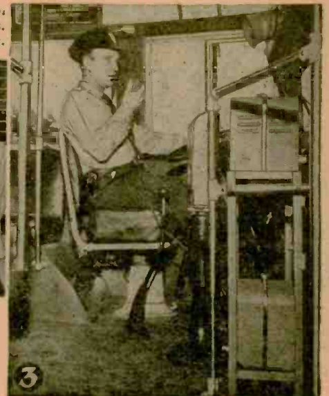
1—A bus driver using new two-way radiophone. 2—Dispatcher's office gets call from a bus. 3—Side view of the bus transmitter-receiver.
